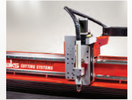
Z-axis carriage automatic lifter with torch height control (THC), magnetic breakaway head, laser pointer and plasma torch
